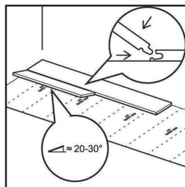
9. Then slide the third plank together horizontally. Slightly lift the plank to be installed by holding your hand underneath. Push the short side joint down gently with your thumb, moving from the inner corner towards the outside until you hear a “click”. Ensure the short side ends are closed by knocking gently on the short side click connection with the palm of your hand or tapping block.
