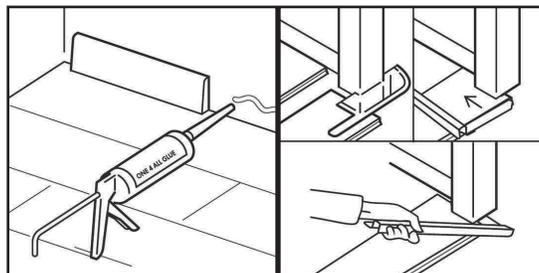
3. If it is difficult to tilt the planks (e.g. under radiators), use a pull bar installation tool to pull the planks together.
