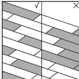
2. Measure the room before you begin installing flooring planks or tiles. Make sure that the last row of panels is at least 3 inches (8 cm) wide when finishing the installation. We recommend snapping a chalk line to ensure a perfectly straight installation.
