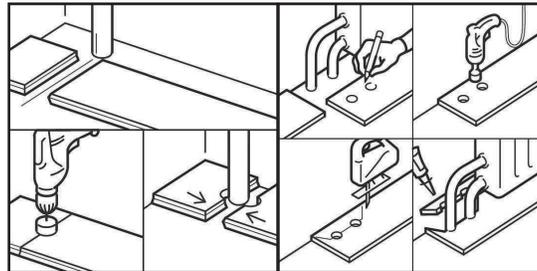
5. For a double pipe, drill a hole equivalent to the diameter of the pipe plus 1/2 inch (13 mm) at each of the marked points. If located on the long side of the plank, make a 45° cut from each hole to the edge of the plank.
